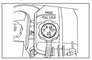
The coolant surge tank and pressure cap are located on the driver's side of the vehicle, toward the rear of the engine compartment. See *Engine Compartment Overview on page 5-14* for more information on location.
